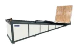
Sanwood Incline impact tester simulates the ability of product packaging to resist shock damage in the actual environment, such as handling, stacking of shelves, sliding of motors, loading and unloading of locomotives, product transportation, etc.
