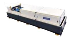
Sanwood Pneumatic Horizontal Shock Response Spectrum Test System that adopts compressed gas energy to provide impact energy, pushes the shock hammer to impact the resonance plate, and generates high energy shock. Compared to traditional pendulum shock response spectrum testers, this machine has the advantages of high energy, stable performance, high reliability, good repeatability, easy adjustment,
