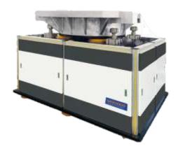
Sanwood Pneumatic Vertical Shock Response Spectrum Test System is used to measure and determine the shock resistance of electrical and electronic products or packaging and to evaluate the reliability and structural integrity of the test product in a shock environment. The shock response spectrum is the total result of a series of single-degree-of-freedom linear systems with different natural frequencies subjected to the same shock excitation response.
