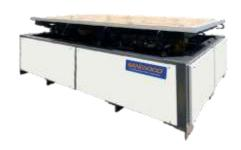
Sanwood brand transportation simulation test system is to simulate the actual road conditions such as shocks and vibrations during the transportation of various items of a specific load and to evaluate the effect of the actual working conditions on the loading, unloading, transportation, packaging, sealing or internal structure of the goods. In order to assess or confirm the products and packaging.
