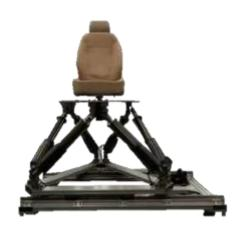
Sanwood 6 DOF simulation tables are closed-loop servo simulation platforms consisting of six servo actuators attached to the upper and lower platforms respectively, and six sets of specialized hinges. Through the telescopic movement of the six actuators, the upper platform can move in six degrees of freedom  $(X, Y, Z, \alpha, \beta, \gamma)$ , enabling the simulation of various space motion attitudes.
