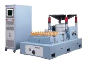
Sanwood vibration testers with dynamic factors such as displacement, velocity, acceleration, and force. Electromagnetic vibration accurately simulates a wide range of conditions that can help improve the quality and reliability of many products.
