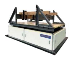
Bounce testing simulates the constant loose cargo state during truck transport. Oftentimes, containers carrying military and civilian hardware (such as medical supplies, electronics, weaponry, and communication devices) travel for extended periods of time and must be transported off-road. All of these items must maintain functionality upon arrival at their destinations.
