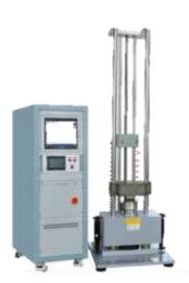
Sanwood brand shock test chambers are specially designed to perform shock and collision tests on products. Although shock tests can be performed with vibration test equipment (shakers), special shock devices are required to achieve high shock values. According to test standards, they can be designed to operate pneumatically or hydraulically, horizontally or vertically.
